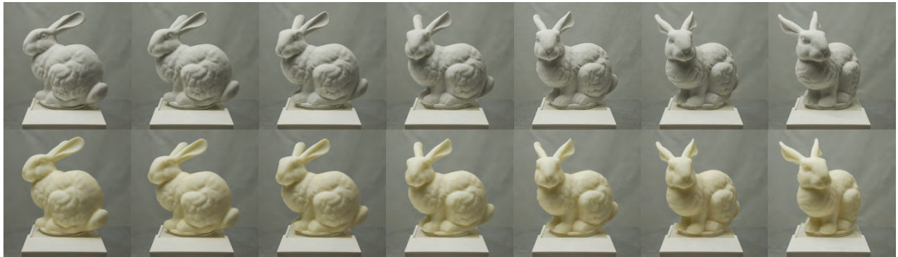
Fig. 5. Experimental conditions of one stimulus. Each shape is printed in two materials and presented in 7 viewing directions. Here we see an example of the Stanford BUNNY printed in ABS shown in the first row. The second row shows the shape printed in SANDSTONE. From left to right we see all seven viewing directions presented in the experiment.
